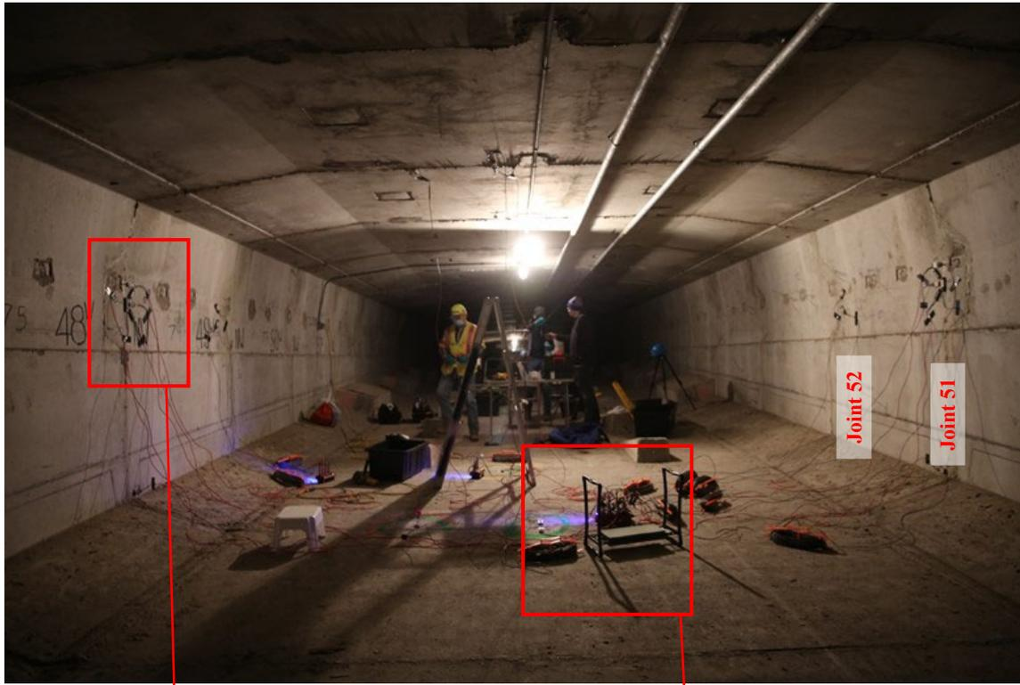
(a) Gauge and Instrumentation layout
