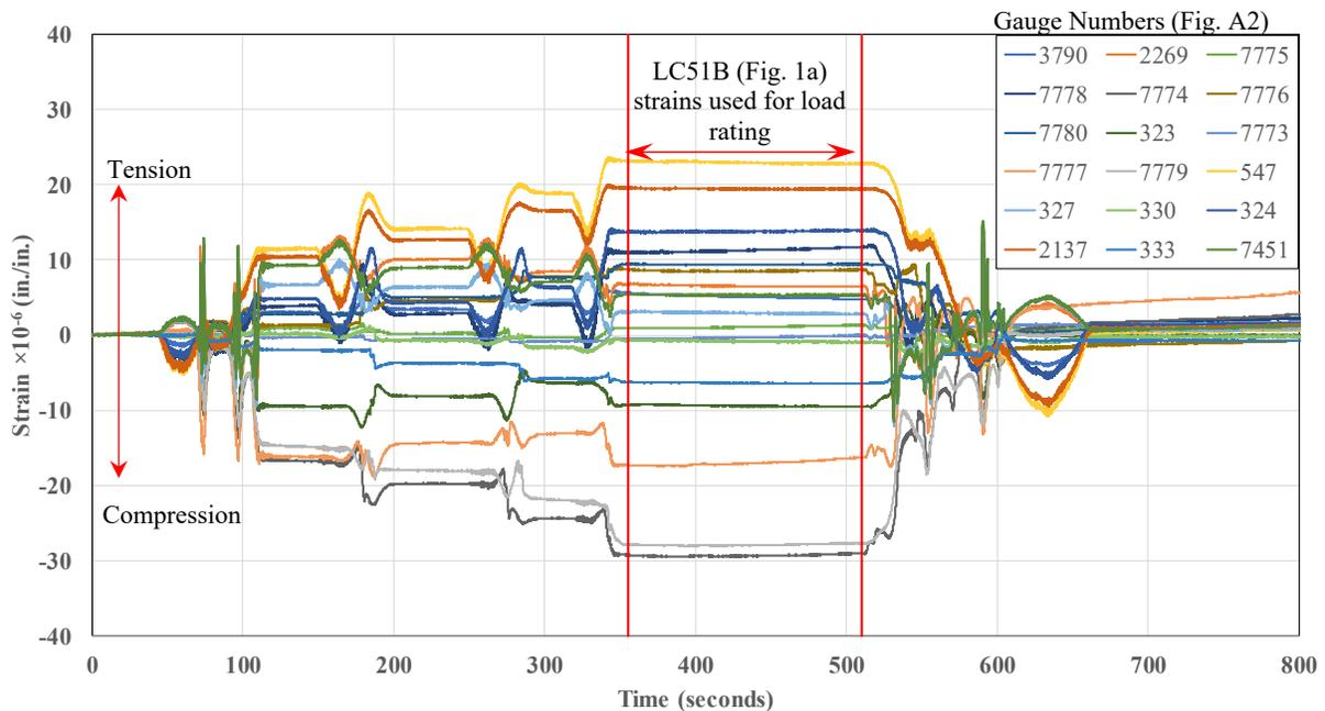
Figure 5: Strains for load case LC51B
