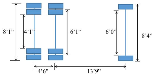
**Figure 4: Load Test Truck Dimensions**
